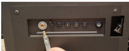
Fig. 21 External pump power connector with matching plug from the external pump
