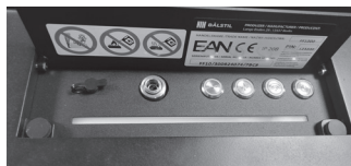
Fig. 9-54 Indication of approximately 5% fuel in the tank
