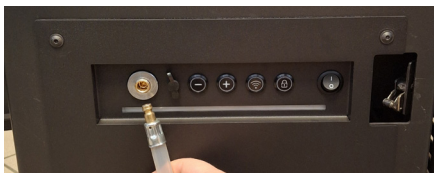
Fig. 20 Fuel filler quick-connect fitting with matching external pump connector
